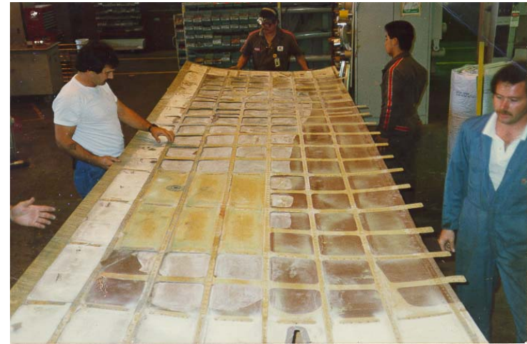
737 body skin waffle doubler with unanodized area
