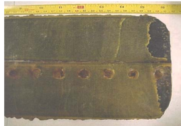
Corrosion products on repair doubler
