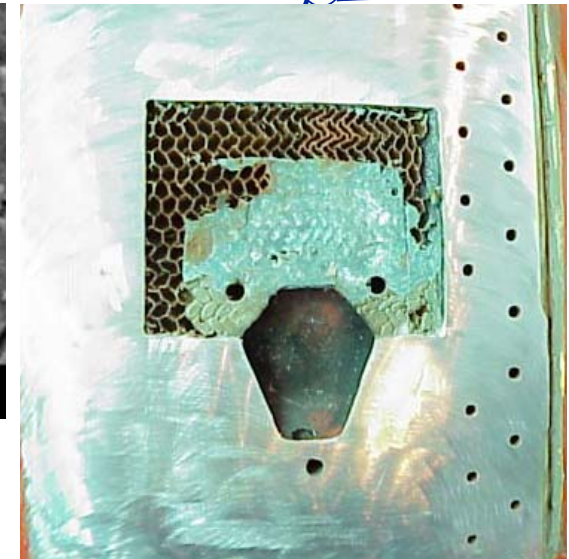
Abraded repair area
